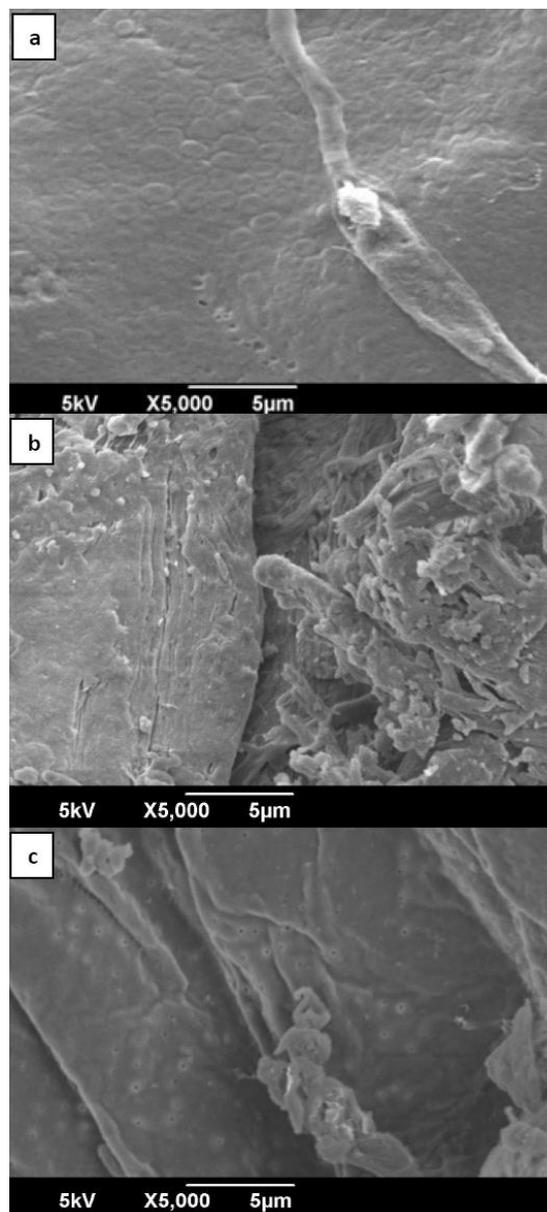
**Figure 2.** The SEM analysis of (a) Papuyu fish scale; (b) Powder of Papuyu fish scale; and (c) Chitosan from Papuyu fish scales
