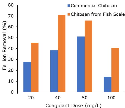
**Figure 3.** Percentage of Iron (III) removed with various coagulant doses (mg /L) of chitosan from Papuyu scales and commercial one.
