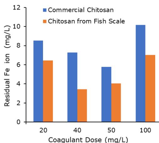
**Figure 4.** Residual of iron (III) using various coagulant doses (mg /L) of chitosan from Papuyu scales and commercial one.
