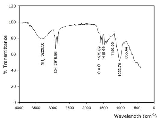
**Figure 1.** FTIR spectra of the chitosan from Papuyu fish scales using solvent concentration of 60% NaOH (% DD of 97.40%)
